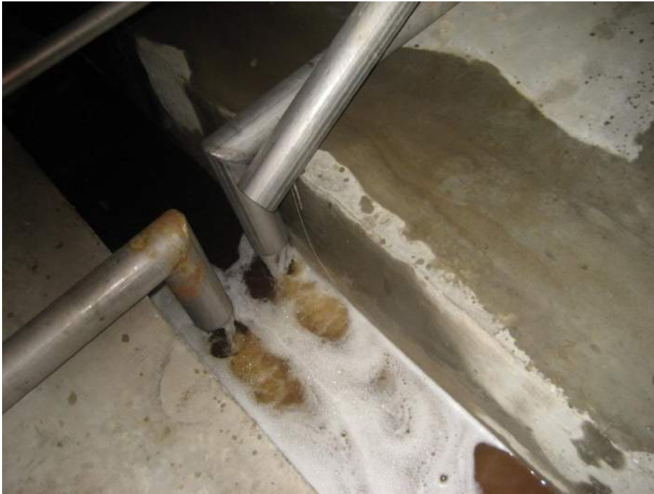
Figure 3-10: Chemical loss by uncontrolled liquor pick-up [22]
