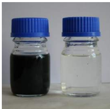
Figure 3-14: Bulk results from membrane filtration: left: washing liquor from CPB dyeing, right: after filtration [27, p. 3]
