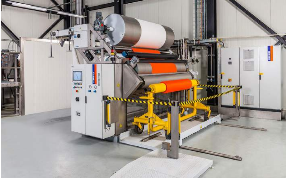
Figure 3-7: Cold pad batch (CPB) dyeing station [24, p. 13]
