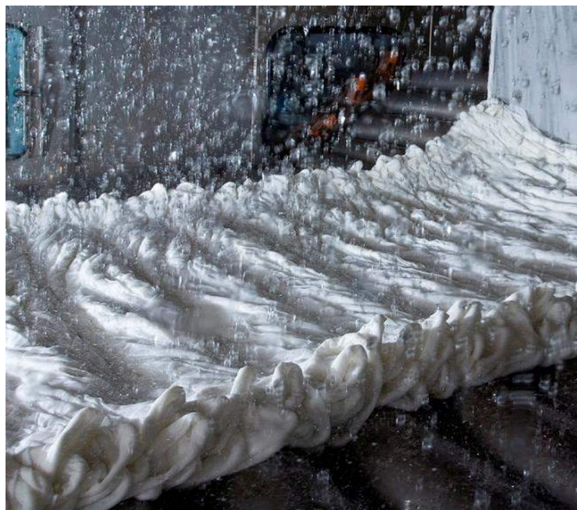
Figure 3-3: Prewash and relaxing of viscose knitwear [23]
