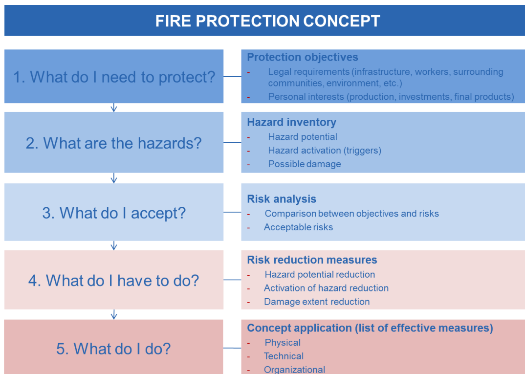
Figure 4-15: Fire protection concept [87]
