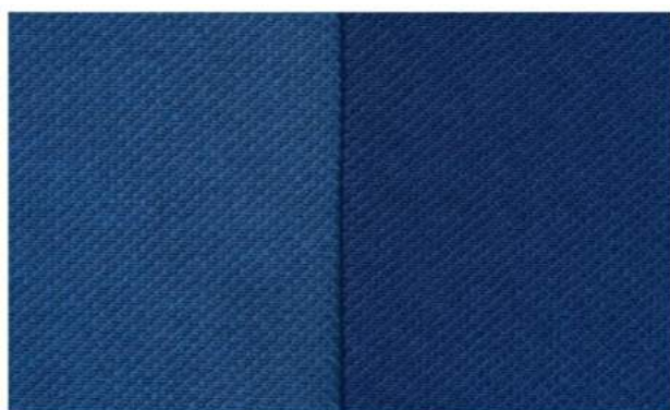
Figure 2-3: Improvement of dye uptake on cotton. Left without mercerizing, right with mercerizing [22]
